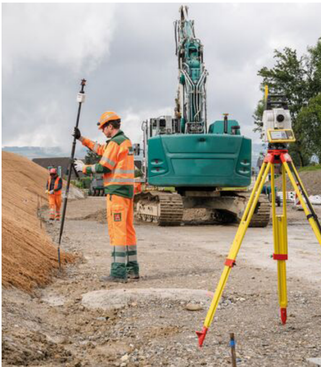
Figure 2: Forget the bubble and increase productivity by measuring points with an arbitrary aligned pole.
