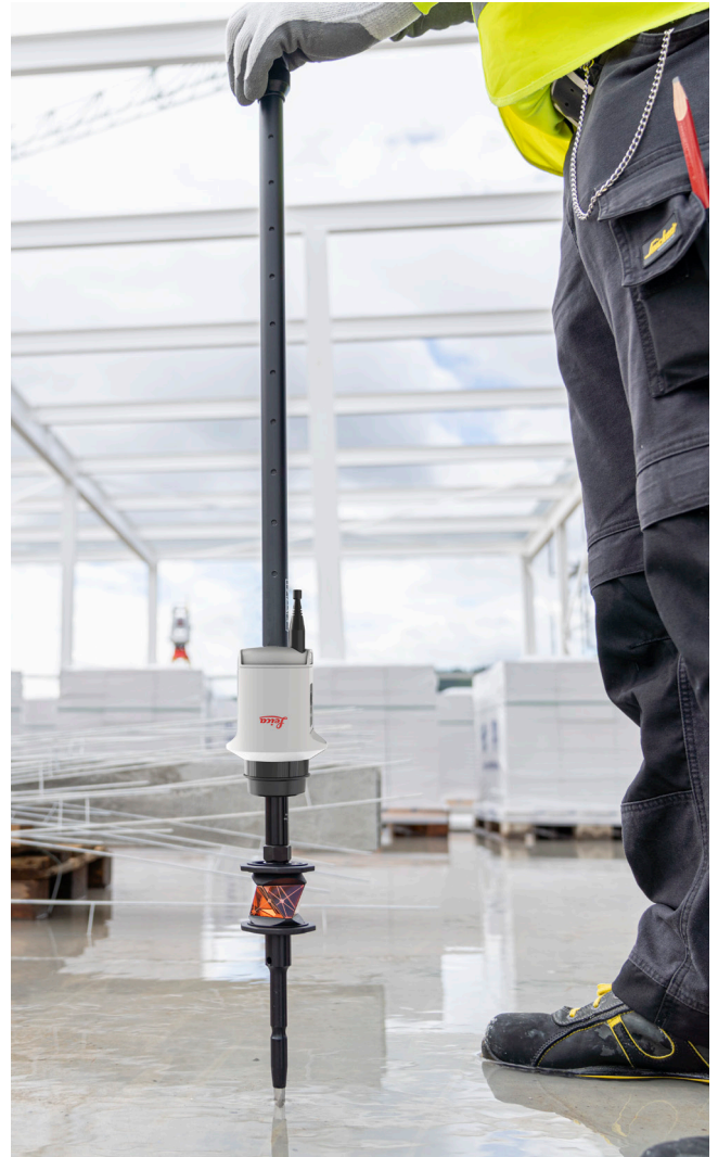
Figure 3: Stake points with highest accuracy in reversed tilt mode by using a small target height.
